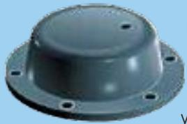
Designed for today's grease-packed systems, the Tamper-Proof Scotseal TF Hubcap features a patented "umbrella" style valve that seals contamination out, yet vents internal pressure as low as 2 P.S.I. The addition of a splash plate to the hubcap design helps protect against the harsh conditions created by road spray, power washers and flooded docks.
